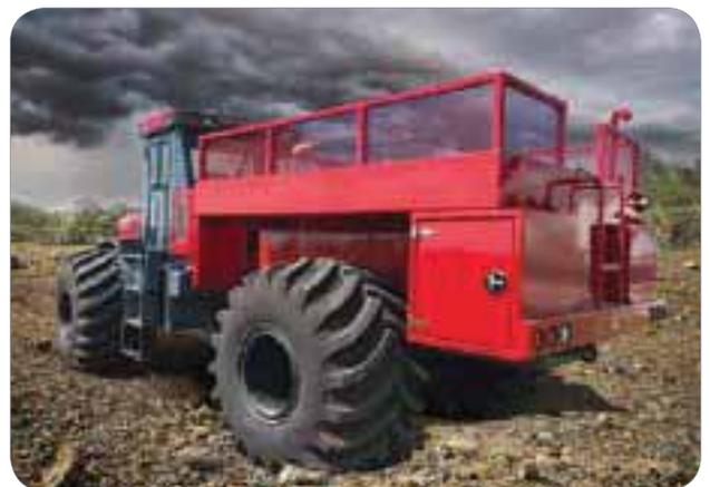
200-horsepower Cummins Tier 4 engine, offers 2- or 4-wheel-drive, and provides a max payload of 28,000 pounds for hauling fuel, water, dirt and more. Top travel speed for each unit is 23 miles per hour.
